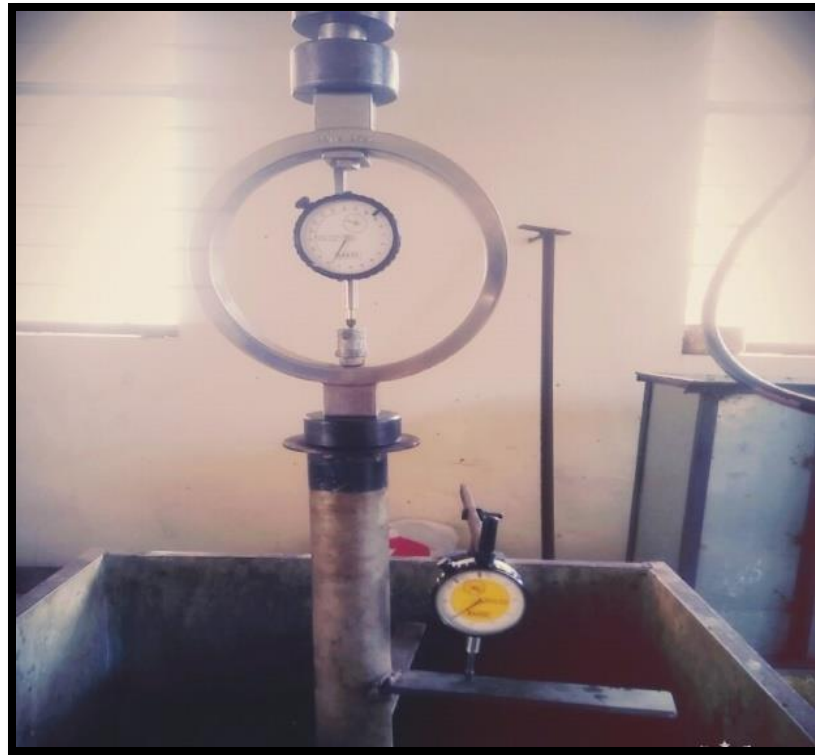
Fig 3 Loading by Mechanical Jack on Footing
